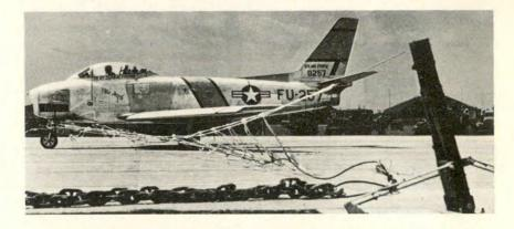
With the arresting cable now positioned and pulled taut, the aircraft begins to drag the heavy, linked chains which are stretched along both sides of the runway.
