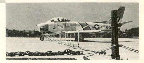
the concrete bases to prevent damage when the stanchion is flattened to the ground. The stanchions can be laid flat when the barrier is not in use.
