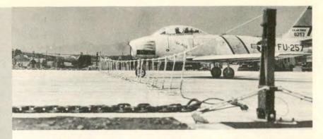
An F-86 moves down the runway and is shown prior to and immediately after initial contact with nylon webbing. Arresting cable will spring up to engage main gear.
